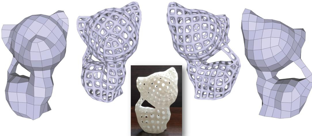
Figure 1: A nearly symmetric quadrangular mesh generated using the operator based representation of vector fields (Azencot et al., 2017) (left and right). The symmetry enables the generation of a very low resolution model, which can be fabricated using additive manufacturing, by thickening the quad mesh edges (left center and right center). The center image is a photograph of the final printed model.
